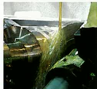
AUTOMATIC SCREW CUTTING
