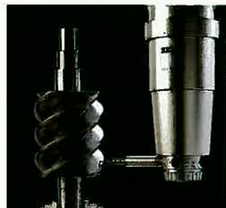
CHECK WITH THREE DIMENSION MEASURING MACHINE
