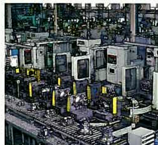
AUTOMATIC PROCESSING OF SCREW CASING
